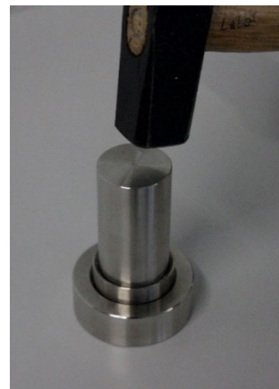
Figure 20: Knock out the sample with a hammer
