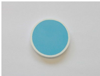
Figure 16: Pressed pellet with a layer of sample
