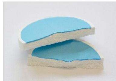
Figure 17: Breaking the sample shows the thin layer
